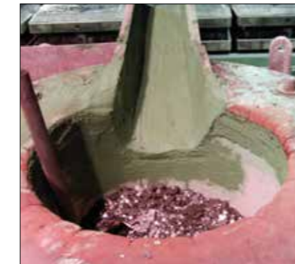
Inductively with starting block or lumpy material
