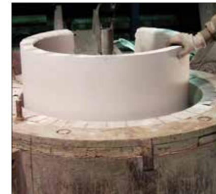
Then insert the DORIT prefabricated crucible by using a lifting device.
