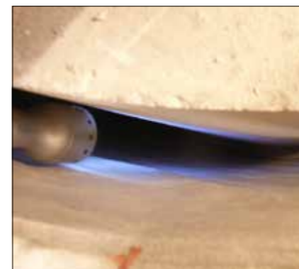
The prefabricated crucible is to adjust in the middle of the furnace
