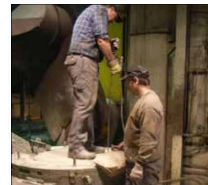
Fix the crucible with backup mix by using a backup mix vibrator.
